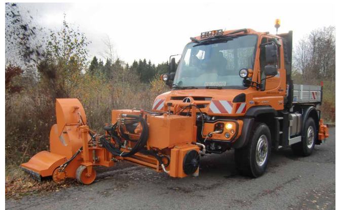
The Unimog from AS Gerätebau with the high-performance BF 600 verge cutter.
