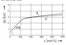
Pressure drop as a function of the **flow volume** D<sub>2</sub> at  $v = 35 \text{ mm}^2/\text{s}$  (0 = casing empty)
