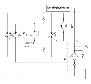
The entire dirt produced in the hydrostatic drive by abrasion is filtered out immediately and is thus not taken in by the pump of the open-loop circuit. This circuit layout is always recommended if the return flow only slightly exceeds the suction flow, i.e. if there is a risk that the 0,5 bar precharging pressure cannot be maintained.
