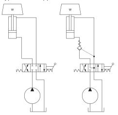
leakage and lock the cylinder in position. Moving the directional control valve to the right sends pressure/flow to the rod end of the cylinder. This pressure also acts on the pilot piston to open the check valve and allow the load to be lowered.
