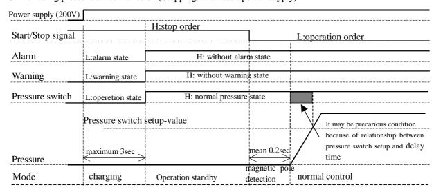
Magnetic pole detection is performed when first starting of motor.
