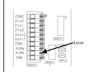
How to connect to the terminal stand board
