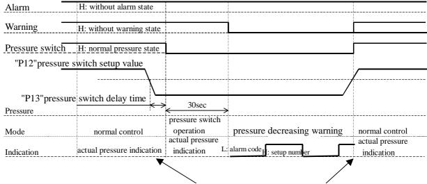
While holding pressure switch operation indication warning code and actual pressure are indicated by turns
