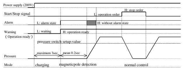
It maybe precarious condition because of relationship between pressure switch setup and delay time.
