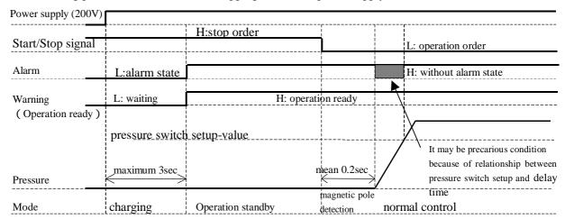
Magnetic pole detection is performed when first starting of motor
