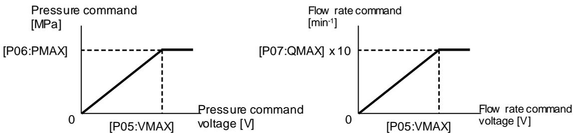
Therefore, adjust the command value relative to each pressure/flow rate setting on the molding machine to ensure linearity, by referring to the table below:
