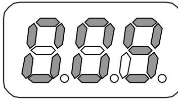
DO4 (1st bit) and DO7 (4th bit) are simultaneously ON.
