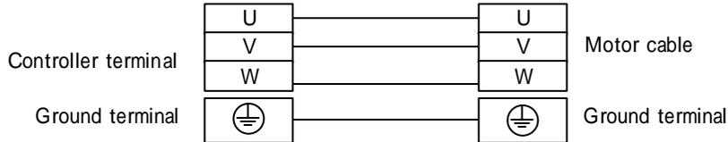
Recommended tightening torque: : 2.4[N · m]
