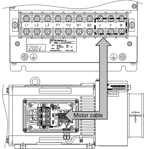
Recommended tightening torque: : 3.5[N · m]
