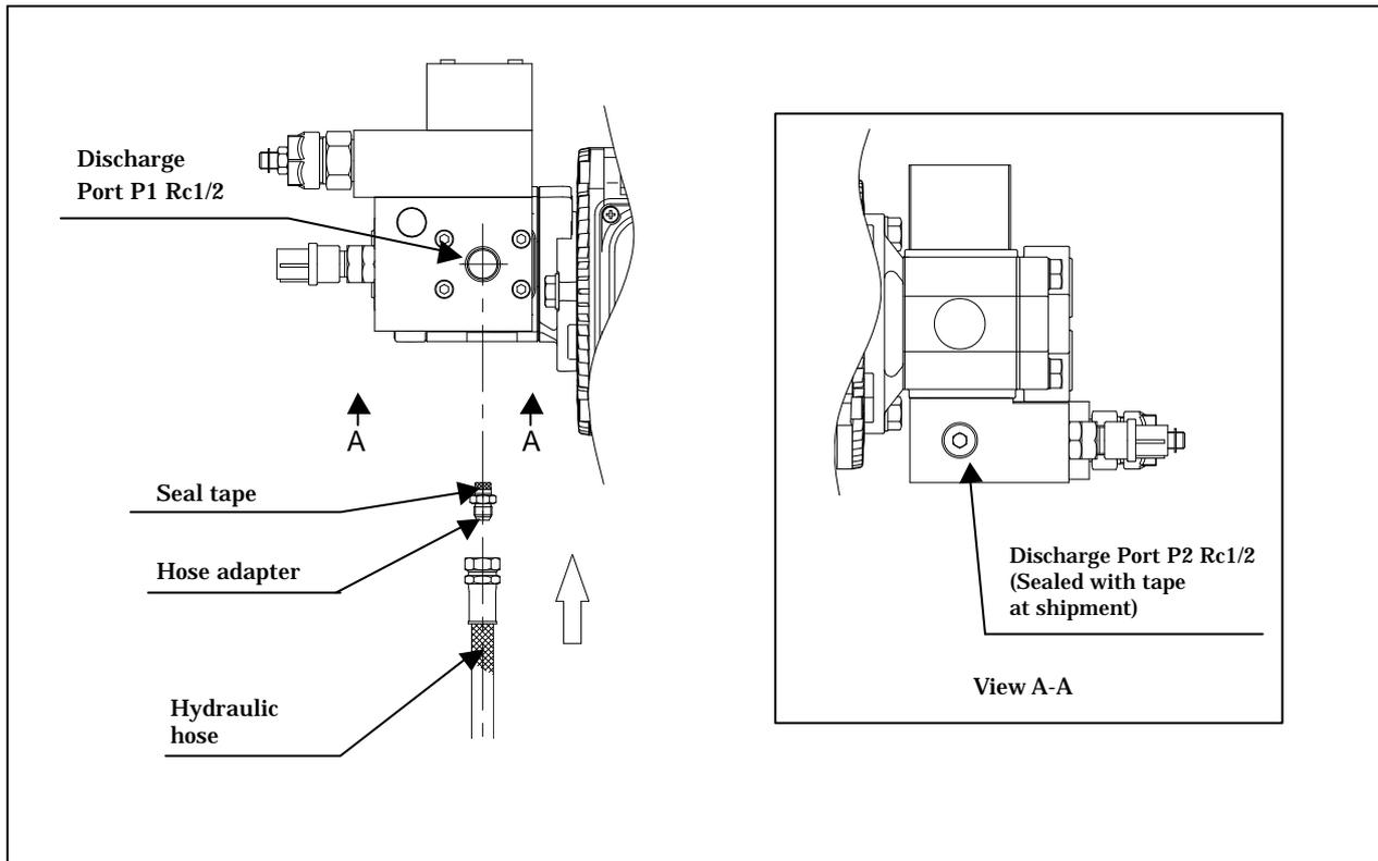
Before shipment, the P1 port has been sealed with a resin plug with O-ring. The P2 port is sealed with a hexagon socket head plug.
