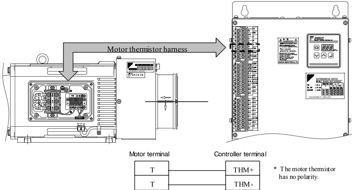
Thermistor connection is included with encoder harness for SUT003018
