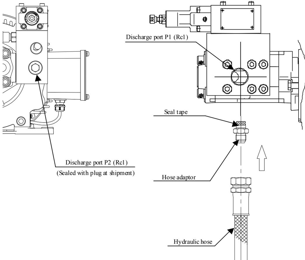
Before shipment, the P1 port has been sealed with a resin plug with O-ring. The P2 port is sealed with a hexagon socket head plug.
