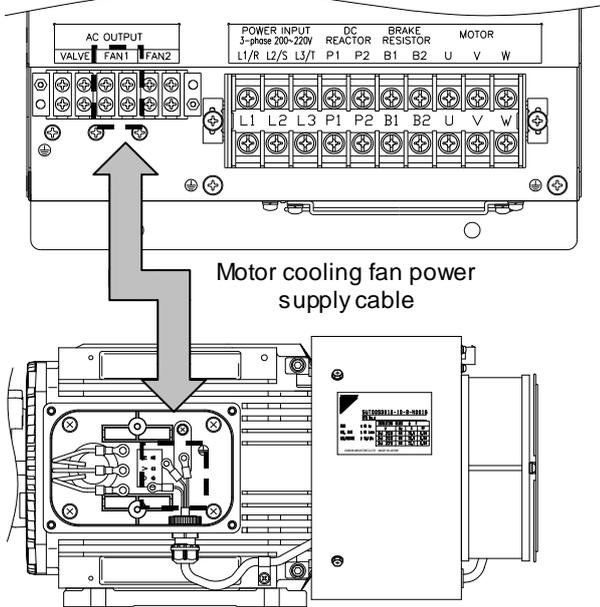
Motor cooling fan power supply cable
