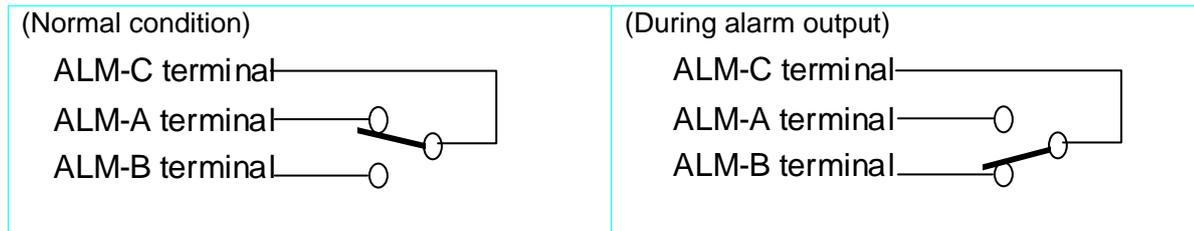
If any of the protective functions is activated, conduct inspections according to the table below to remove the cause of the alarm and take corrective actions.
