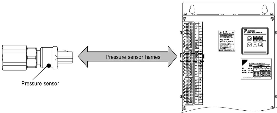
The pressure sensor mounting position varies depending on the unit model. Refer to “3.5.1 Motor pump outer dimensions”.
