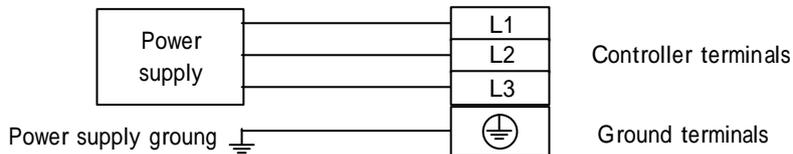
Recommended tightening torque: 2.4[N · m]
