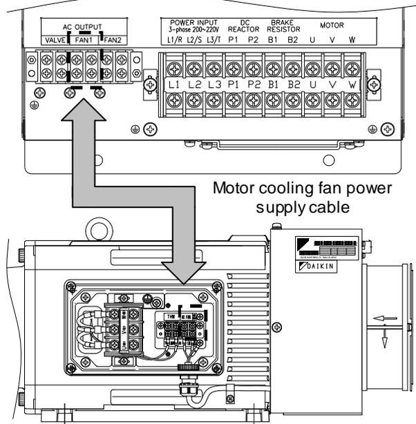
Motor cooling fan power supply cable
