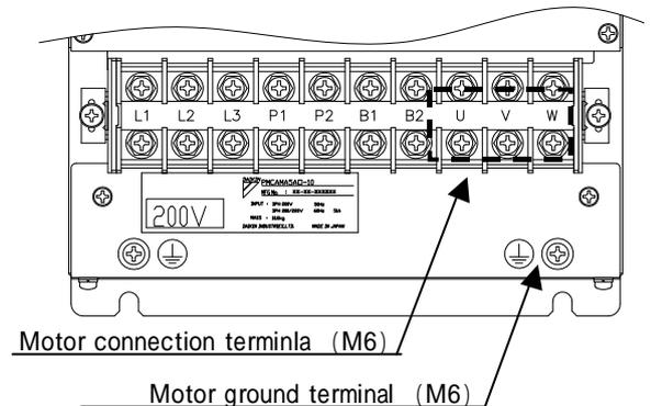
Recommended tightening torque 3.5[N · m]
