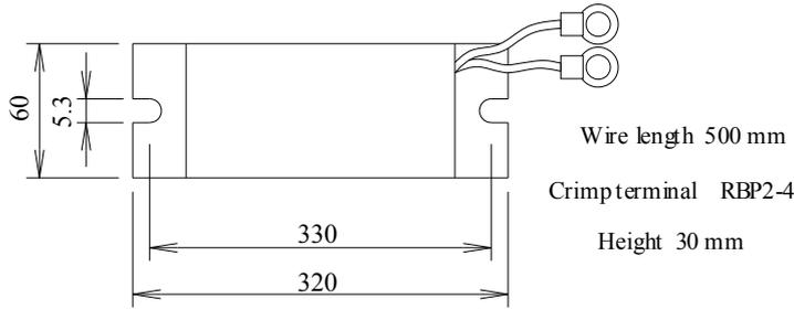
To use the above regenerative braking resistor, connect the specified number of resistors in parallel.
