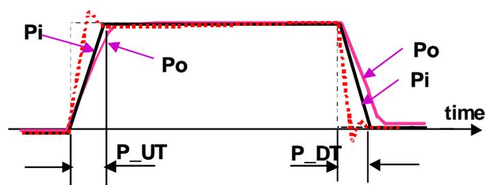
For the pressure rising time constant, specify a time required to increase a pressure command from "0" to "P06: PMAX".
