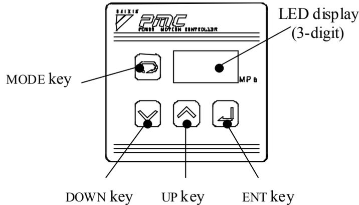
The controller provides a 3-digit, 7-segment display and four key switches, as shown on the left. In the normal mode, the display indicates a current pressure value (MPa).
