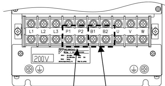
DC reactor connection terminal (M6)
