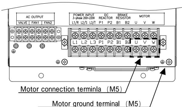
Recommended tightening torque 2.4[N · m]
