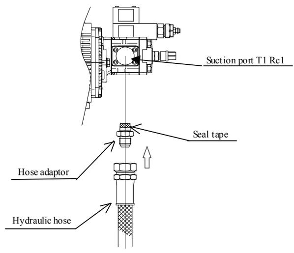
Before shipment, the suction port has been equipped with a cover port. Remove the cover port, and connect the hydraulic hose. Tighten the hose by winding seal tape. For piping to the suction port, provide an approx. 150-mesh suction filter.
