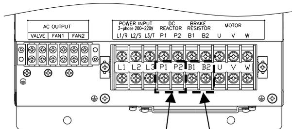
DC reactor connection terminal (M5)
