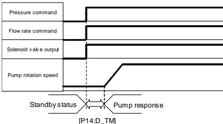
If the pump makes response upon rising of the command voltage from the standby status, the pump starts up before switching operation of the solenoid valve in the hydraulic circuit is completed. This may cause an abrupt change in pressure and flow rate, resulting in a shock as “Po” and “Qo” shown on the right.
