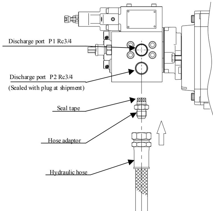
Before shipment, the P1 port has been sealed with a resin plug with O-ring. The P2 port is sealed with a hexagon socket head plug.
