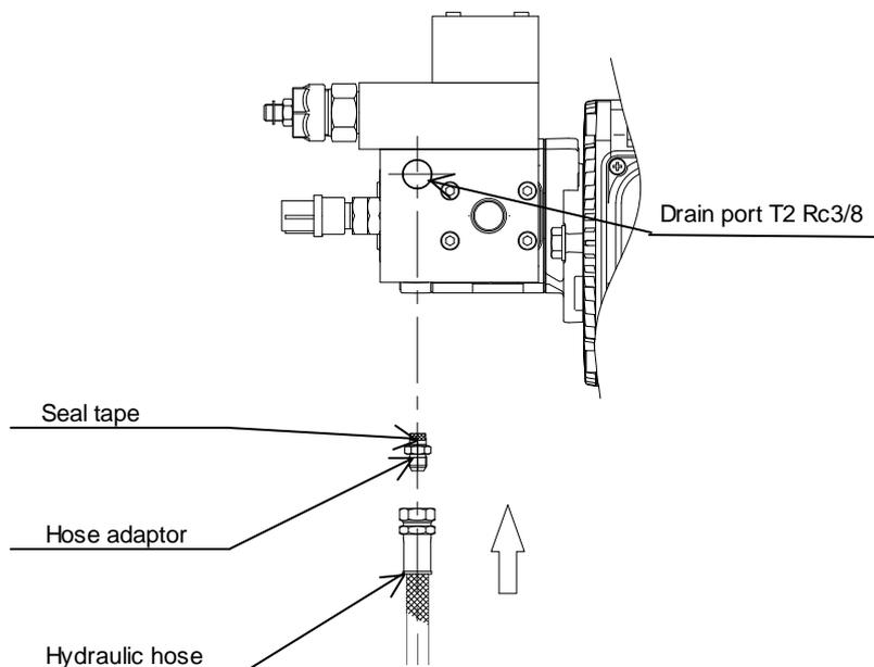
Before shipment, the T2 port has been sealed with a resin plug with O-ring.
