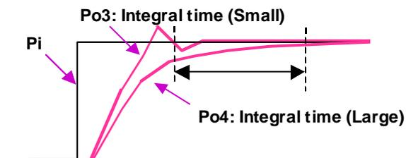
As described above, when the proportional gain setting is large and the integral time setting is small, a response time relative to a command is shortened, but operating condition easily becomes unstable (e.g. hunting occurs.) because the amount of correction becomes large. While monitoring actual operating conditions, change the proportional gain and integral time settings, to adjust the response time and stability.
