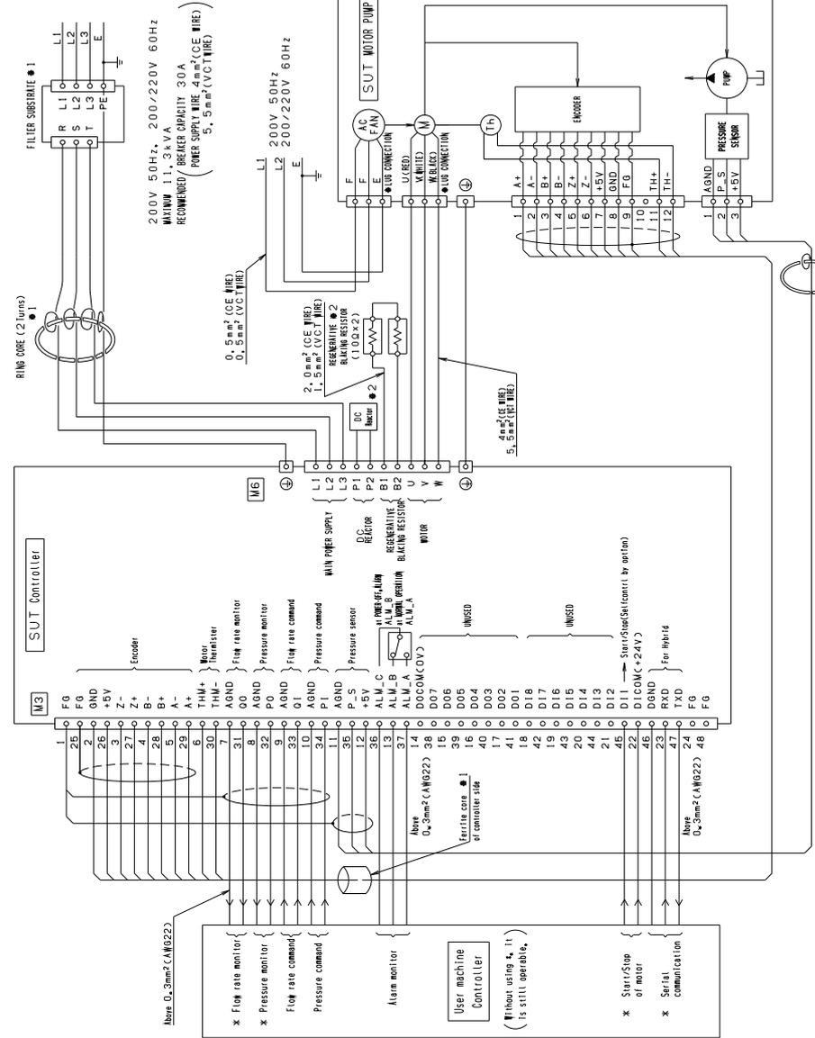
SENSOR HARNESS SPECIFICATION (The length must be within 5m when manufacturing)
