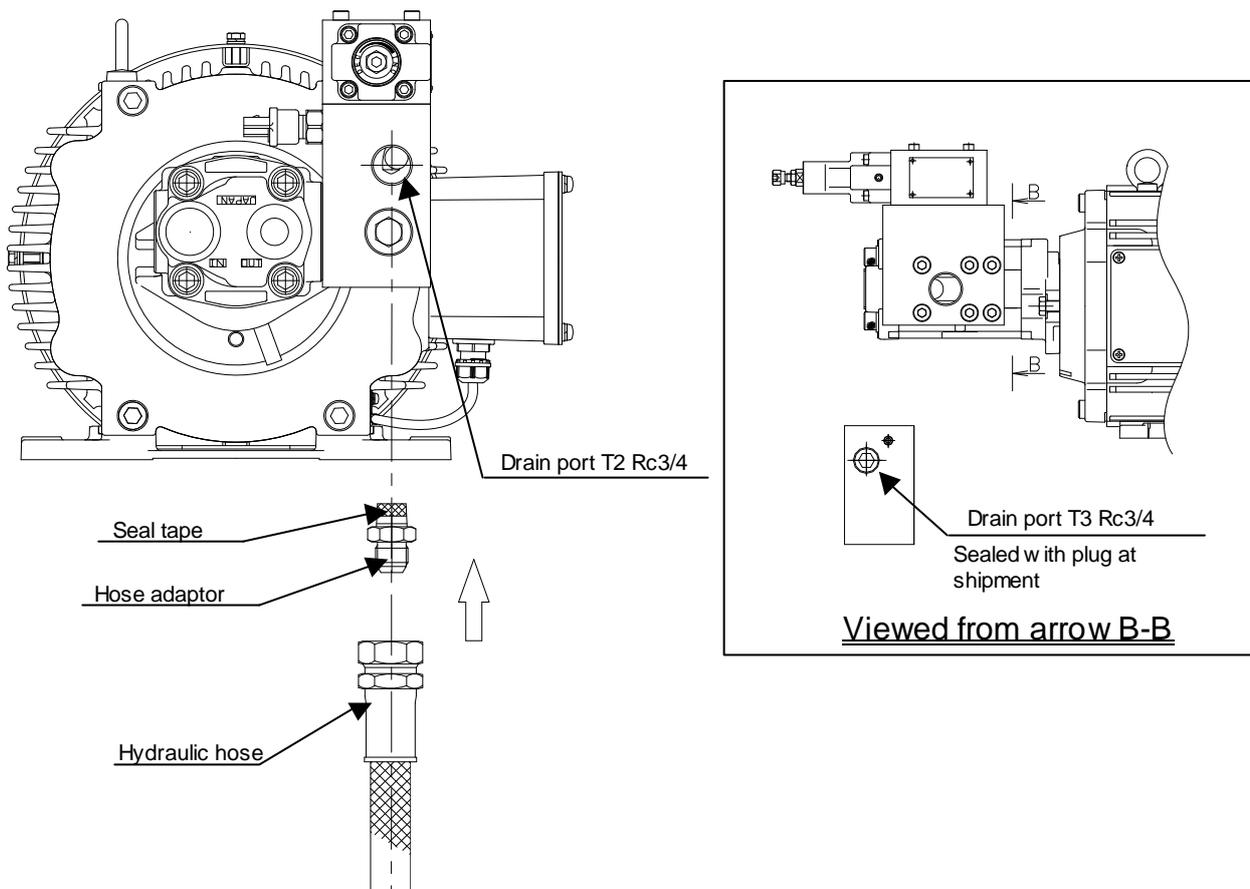
Before shipment, the T2 port has been sealed with a resin plug with O-ring. Remove the resin plug with O-ring, and connect a hydraulic hose. Then, tighten the hose by winding seal tape.
