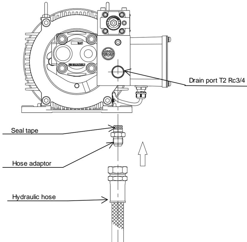
Before shipment, the T2 port has been sealed with a resin plug with O-ring.
