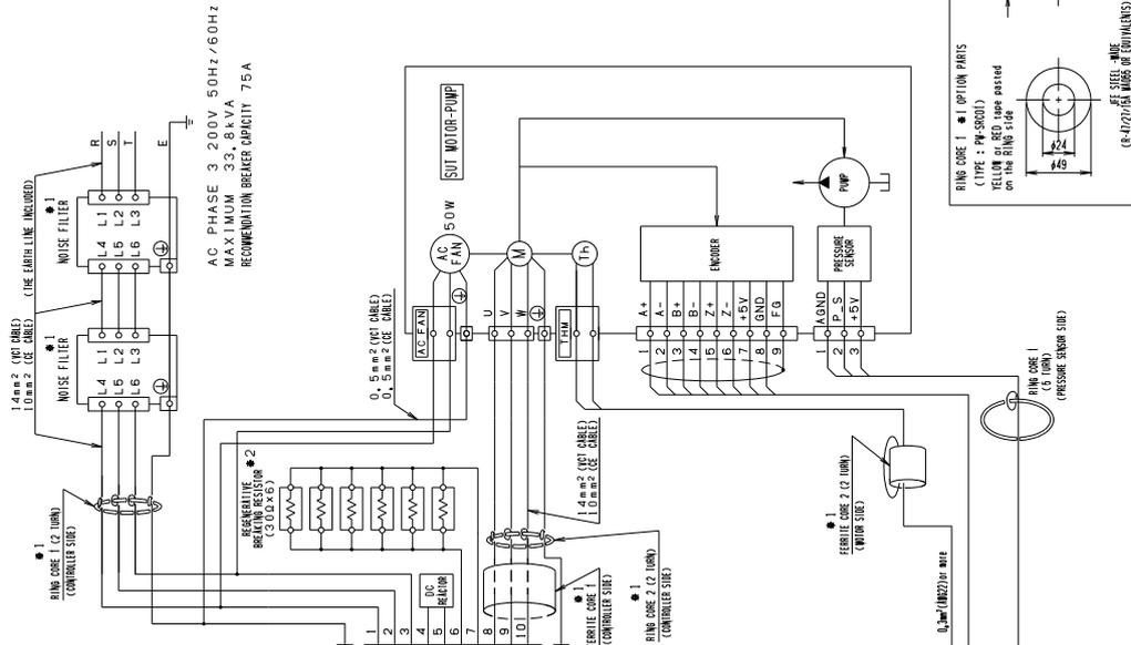
SENSOR HARNESS SPECIFICATION (The length must be within 5m when manufacturing)
