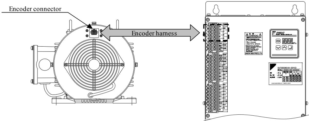
1) Prepare the encoder harness, crimp terminals, connector and dedicated wiring tool.
