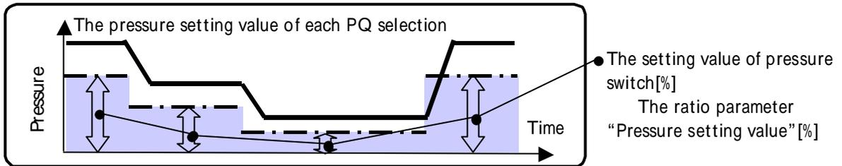
Pressure switch working example
