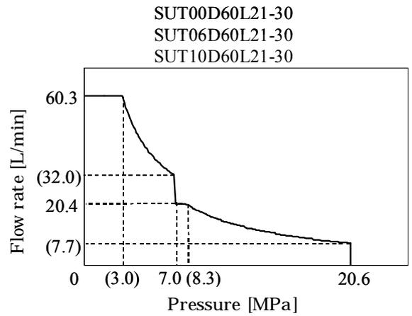
\*1 The above charts show the typical characteristics when the oil temperature is 40 °C.
