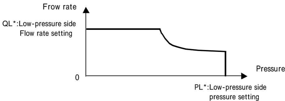
\* Please refer to "12.3.3 [P40: PL\_D] Settings when operating only at high pressure side (single) " for more information about how to set the high-pressure and low-capacity operation.
