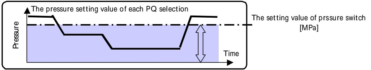
Pressure Unit : the setting value of "P08 : Alarm output mix" is "2"
