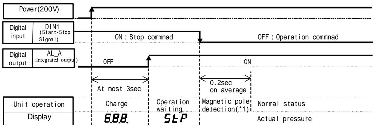
\*1 Magnetic pole detection is performed only when the motor start at the first time after turning on the power.
