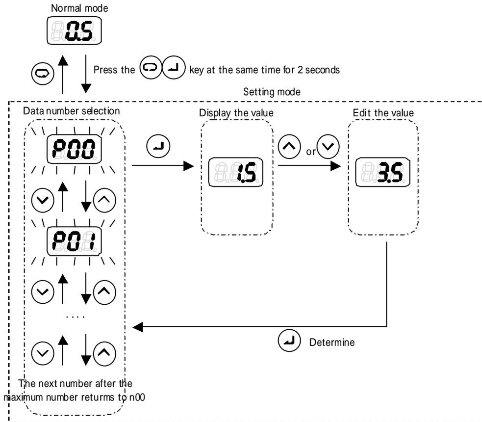
Press the at the same time in normal mode. It will switch to setting mode after about 2 seconds.
