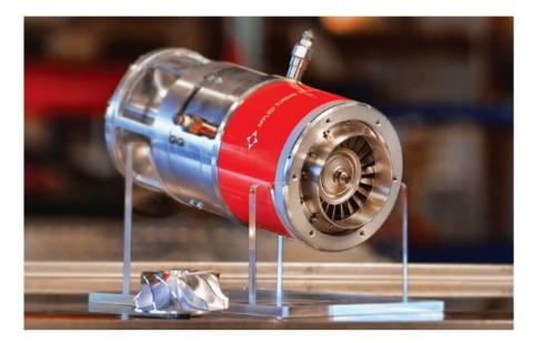
Drying streets requires moving heated air rapidly over the pavement. Leaders at Applied Turbine Technologies immediately recognized the potential of diesel-powered micro-turbines, which are about the size of large coffee cans, to provide an alternative to the propane-based driers. Each microturbine can create airflow of 50 cubic meters per minute at up to 650 degrees Celsius (1200 degrees Fahrenheit).
