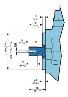
Splined ANSI B92.1a-1976 Pitch 16/32" DP Pressure angle 30° Tolerance class: 5
