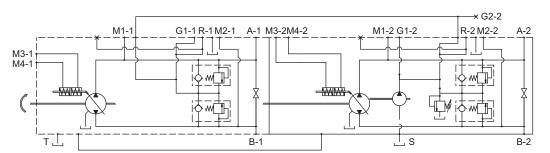
Ports T and G of the first pump must be connected with ports T and G of the second pump.
