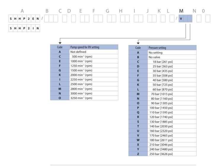
For pressures higher than 210 bar [3046 psi] and lower than 40 bar [580 psi] apply to your Turolla representative.
