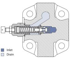
Integral relief valve schematic (external drain)
